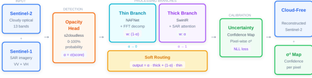
Figure 3: Dual-branch cloud removal architecture with opacity-based soft routing.
