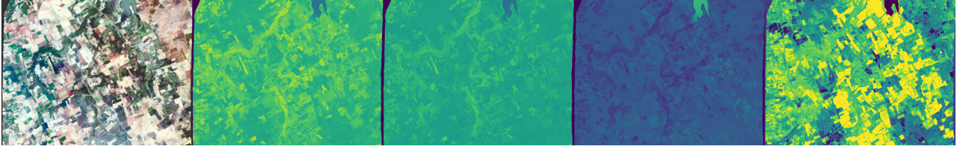
Figure 6: Multispectral indices computed from the AVIRIS-NG aerial images. From left: true color approximation, NDVI, NDRE, HDWI, and TCARI/OSAVI. Brighter colors indicate higher index value. Note that TCARI/OSAVI properly identifies region’s dry vegetation, and HDWI discerns the lake near the top of the image.
